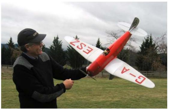
Chilton from 1949 Aeromodeller plan scaled to 42 inch span and powered by the ubiquitous Cox BabBee tuned and proped for long engine runs.
