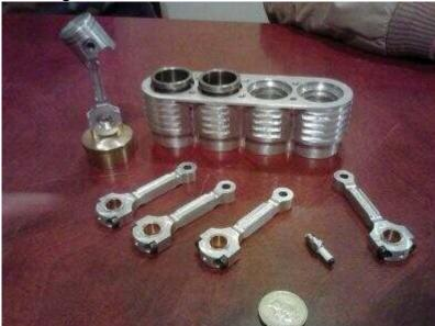
Brent Coburn has been making the con rods for his 4 stroke marine engine – profile was cut out with high pressure water jet cutter and then machined. He has made the pistons and the cylinders, which have been modified for water cooling, are under construction. Cylinder liners are made from cast iron. Cylinder heads and valves being machined. Using commercial miniature spark plugs ex-China with ignition CDI unit being considered to replace conventional distributor.
